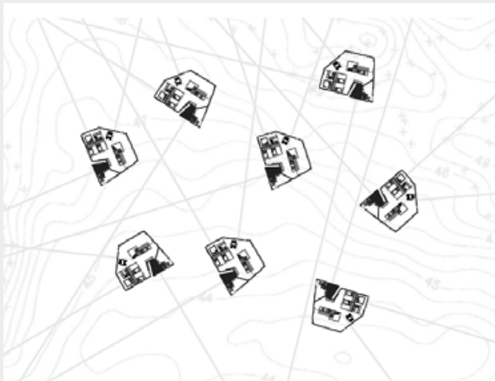
Non-conflicting sight lines
